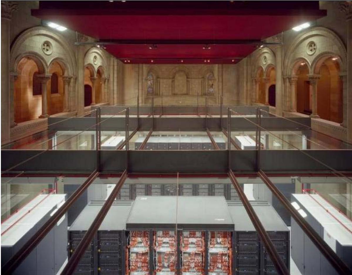
MareNostrum Cluster in Barcelona. The central Myrinet-2000 switch has 2560 host ports. Photo courtesy of IBM.
