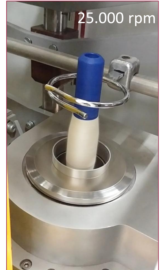
Cryostat 2.0 (65 K, max. 50.000 rpm)
