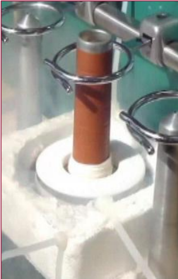
Test in offenem LN 2 (~10.000 rpm)
