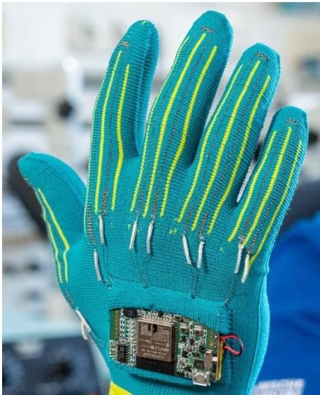
Figure: Left: Sensor glove with fully integrated textile sensors and processing unit Right: 60GHz receiver ASIC with bondwire antenna [1] © IEEE
