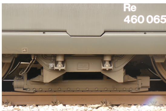
(c) Permanentmagnetschienenbremse (PMB)
