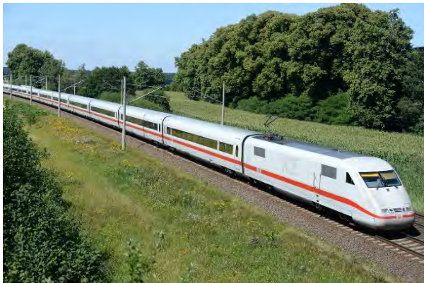
ICE: c_w = 1,55 ICE-Triebkopf: c_w = 0,21
