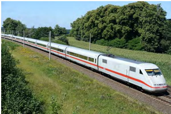
ICE: c_w = 1,55 ICE-Triebkopf: c_w = 0,21
