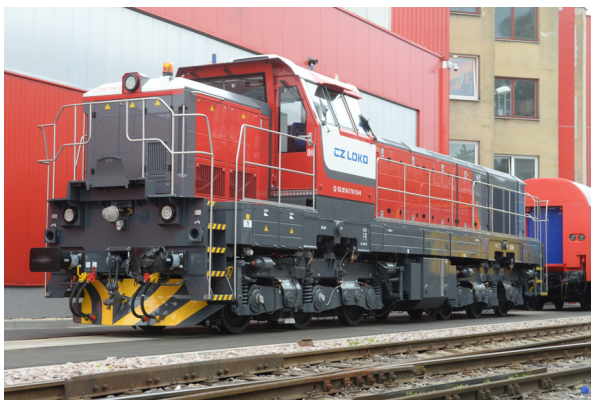
(b) Lokomotive CZ Loko EffiShunter 1600, Ansicht 1
