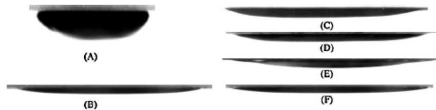
Fig. 8. Digital image of sessile oil drops on a quartz substrate, in brine with different NaOH concentrations, at equilibrium state and ambient temperature. (A) 0; (B) 0.1 wt%; (C) 0.2 wt%; (D) 0.3 wt%; (E) 0.4 wt%; (F) 0.5 wt%.
