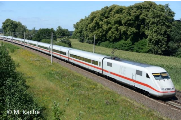
ICE: c_w = 1,55 ICE-Triebkopf: c_w = 0,21
