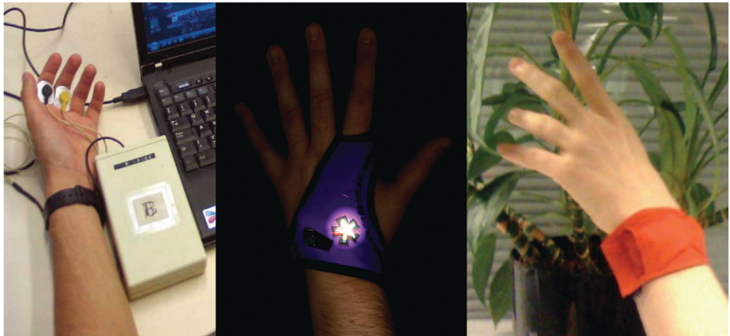
Abbildung 1: electrodermal activity sensors [4, S. 3]
