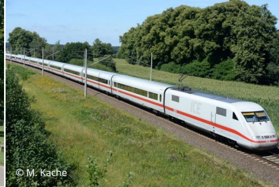
ICE: c_w = 1,55 ICE-Triebkopf: c_w = 0,21
